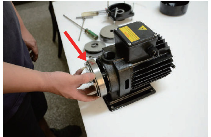
Step3: put the chamber in it
