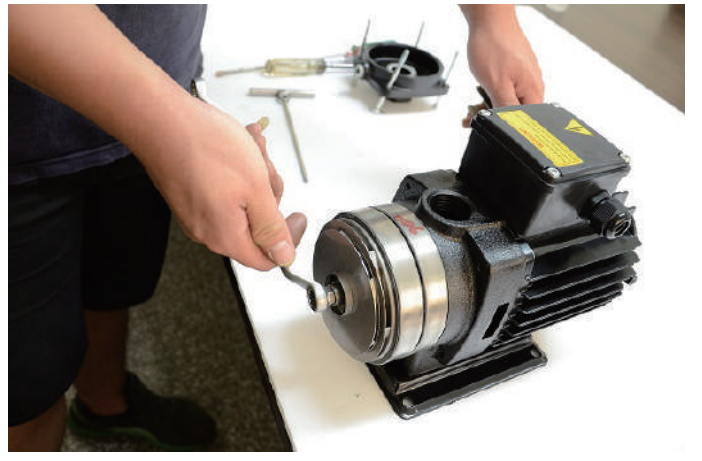
Step9: put the lock nut in, grasp the universal pliers, use box wrench lock the lock nut
