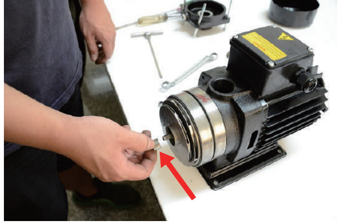
Step7: put the sleeve in it
