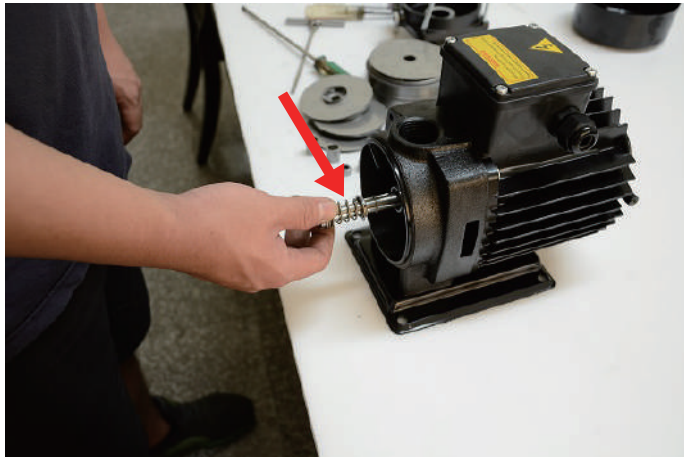
Step2: put the spring in it
