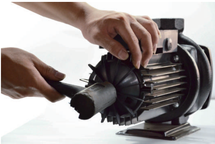
Step10: use hammer to beat the fan in it
