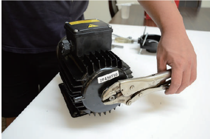
Step8: use universal pliers to grip the end of motor spindle
