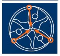
**Photo caption:** On the GARANT MasterSteel FEED solid carbide drill, the self-centring forces act on three cutters instead of just two.
