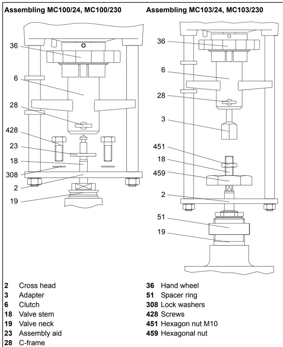
**diagram 6** Mounting the linear actuator on the valve
