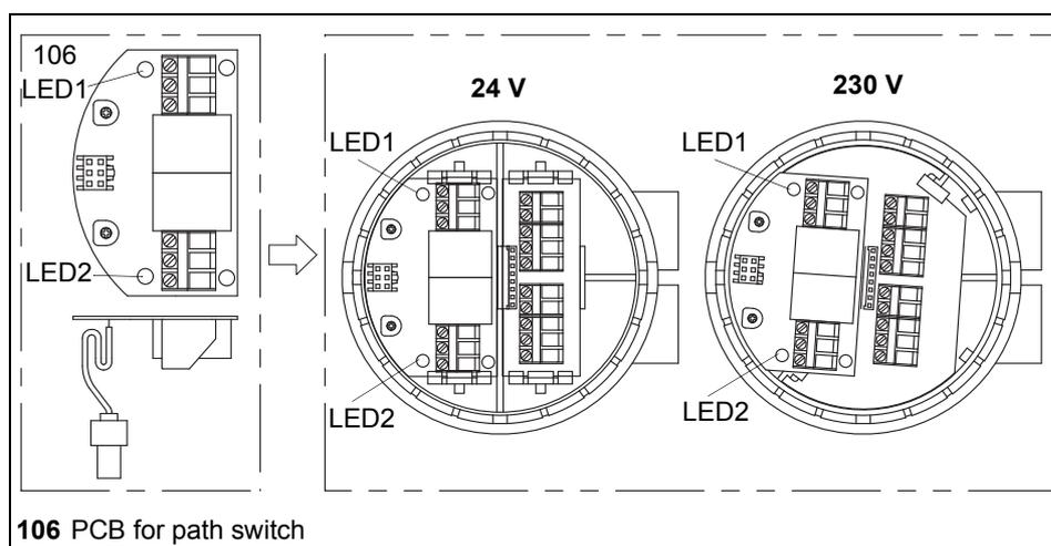
diagram 3 Position switch PCB in cover
