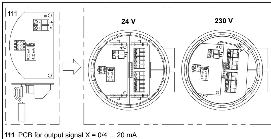
diagram 2 PCB for mA output signal in cover
