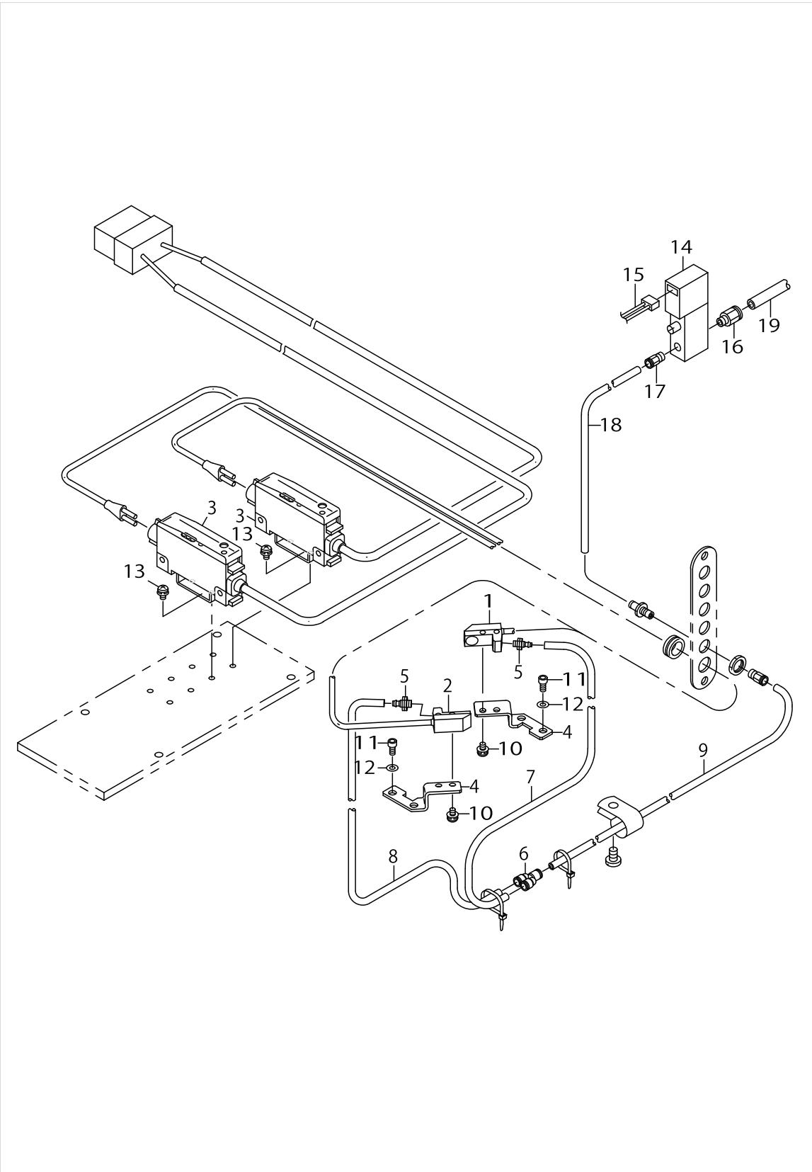
BOBBIN THREAD REMAINING AMOUNT DETECTING DEVICE
