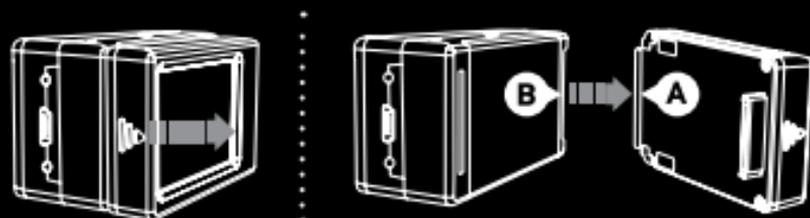
1. Pull back on left side of BacPac marked with the arrow to disconnect from the HERO bus port.
