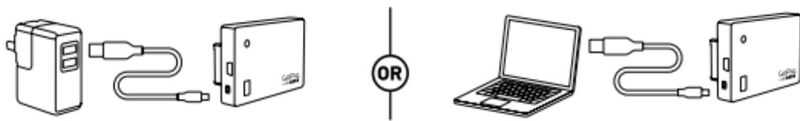
For fast charging, connect the Battery BacPac to a USB wall charger (sold separately). You can also charge the Battery BacPac by connecting it to your computer using the included USB charging cable.
