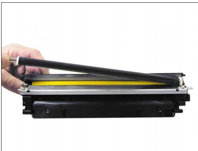
12. Slide the developer roller over and remove.
