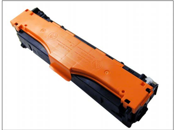
27. Install the drum cover on to the cartridge. Spread the two halves apart slightly so it fits properly.
