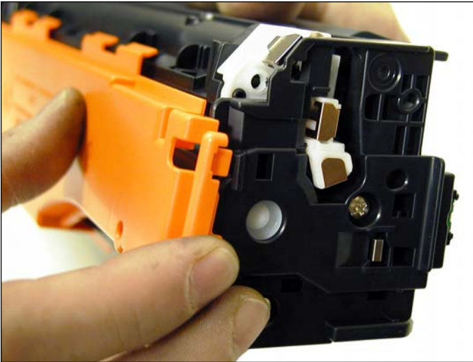
27. Install the drum cover on to the cartridge. Spread the two halves apart slightly so it fits properly.
