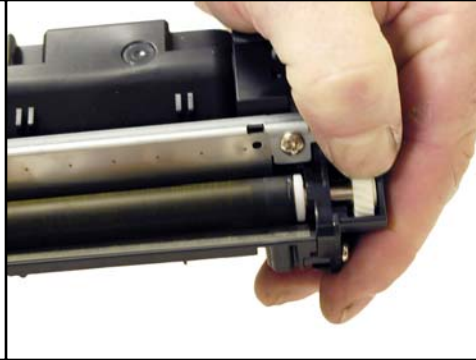
22. Install the gear end cap and screws. Turn the developer roller so it mates properly with the drive gear. Make sure the spring arm works!
