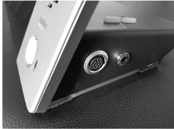
Talk-Button | MiniCON Mic Interface | Head Phone socket | Volume Control
