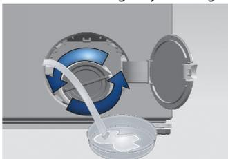
a Pull the emergency draining hose out from its seat
