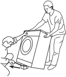
Tilt the machine backwards to remove the packaging reinforcement. Remove the packaging reinforcement by pulling the ribbon.
