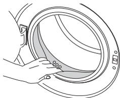
After every washing check that no foreign substance is left in the drum. If the holes on the bellow shown in the figure is blocked, open the holes using a toothpick.
