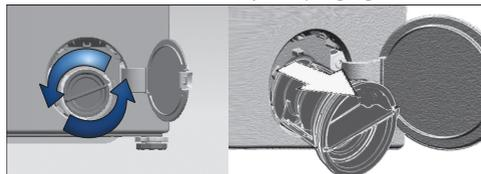
d Turn the pump filter to take it out.
