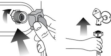
1. Tighten all hose nuts by hand. Never use a tool when tightening the nuts.
