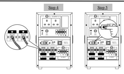
5. Connect the batteries to the BATTERY INPUT. (Step4)
