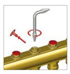
Starting from a totally closed position, open the lockshield according to the enclosed chart, in order to achieve the desired flow rate. The adjustment has to be done by means of a hexagonal key in the size of 6 mm.
